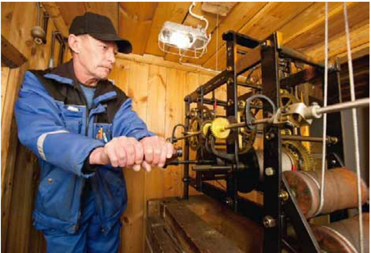
Winding up the clock in the Jetty Barracks tower is part of the job of maintenance man Jorma Hiltunen. The latest renovation of the clock machinery was undertaken in 1979 by precision mechanics students at the Westend Vocational Institute for the Disabled.
